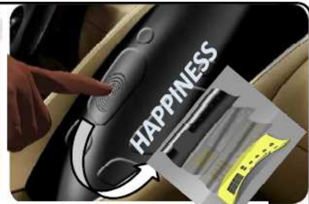
Haptic feedback on reconfigurable touch sensing area in active mode
