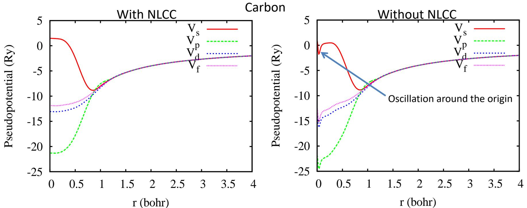
Even when the overlap between core and valence charge density is small, a small NLCC helps to eliminate the pseudopotential wrinkles for small value of the radius.
