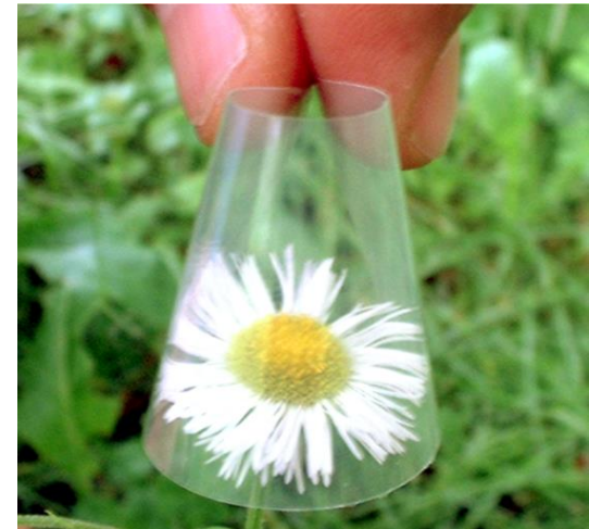
Flexibility and transparency of acrylic resin film with 60 wt% BC nanofibers
