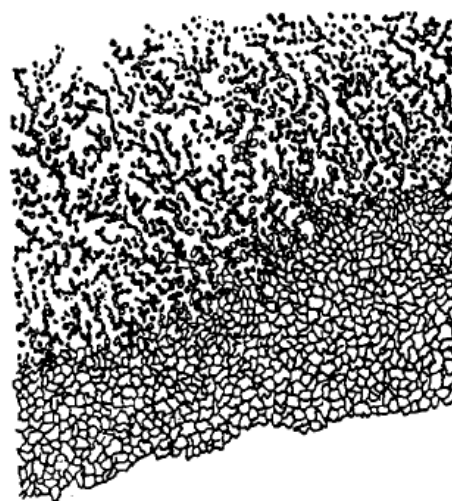
Figure 1: The solidification wave front is a traveling fractal cluster of aggregated microspheres of the solid phase of the solvent ( \text{H}_2\text{O} ) distributed in the surface layer of the solution. The dimensions of the nuclei of the solid phase during their evolution vary from 0.1 to 10 microns. The motion of the crystallization front is directed from the bottom to the top.
