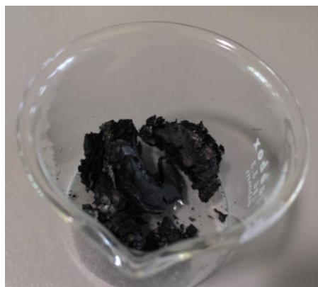
Figure 1: Graphene aerogel. AIMPLAS.
