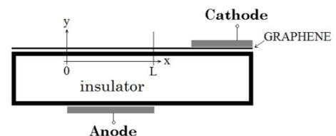
**Figure 1:** Cross-section of the vertical MIGM diode considered in this work.
