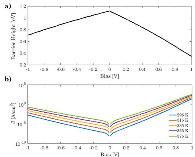
**Figure 2:** a) Schottky barrier height for electron transport and b) Current density –voltage ( $J$ - $V$ ) curve of a MIGM diode for different temperatures.
