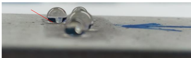
Figure 1: Superhydrophobic behaviour (CA above 160°) of the developed transparent nanocoating applied on mortar specimen, after 40 cycles of abrasion test.
