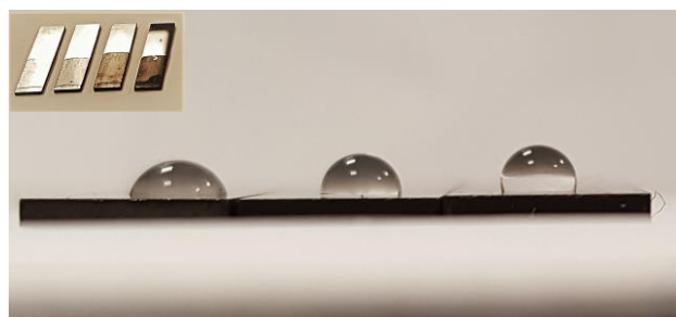
Figure 2: Different thickness of polymer graphene nanoplatelets films in glassy carbon electrode substrate (GCE). DI water has been dropped on the surface to prove the increase of the thickness using the Layer by Layer method. The inset photo corresponds to 2, 5, 10 and 20 layers of the nanocomposite, where the increase of the thickness is visual.
