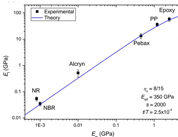
**Figure 2:** Variation of  $E_f$  with  $E_m$  for the M25 GNPs reinforcing a series of polymeric matrix different materials with different values of matrix modulus,  $E_m$ . The solid line is the behaviour predicted with the parameters indicated.
