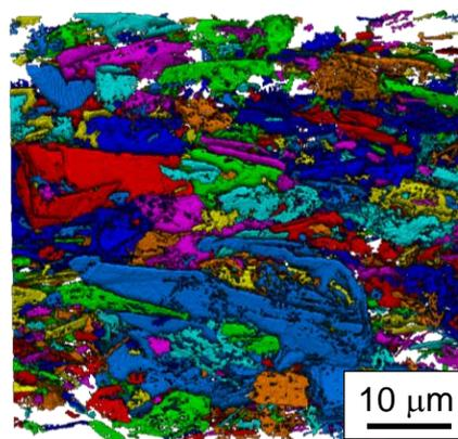
**Figure 1:** Artificially-coloured image of a CT scan of a natural rubber nanocomposite [2] containing M25 GNPs nanoplatelets.
