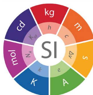
Figures : a) The revised SI based on fundamental constants. b) Hall resistance ( R_H ) and longitudinal resistivity ( R_{xx} ) as a function of the magnetic flux density in a Hall device based on CVD graphene on SiC (GaAs/AlGaAs device for comparison)
