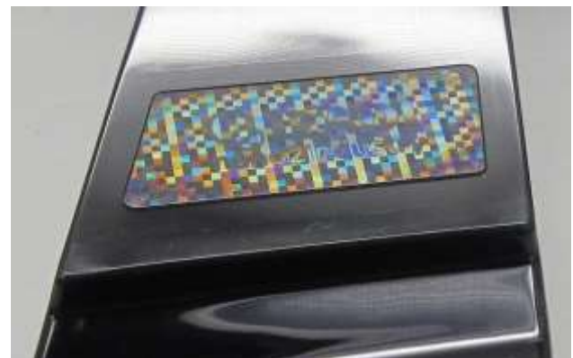
Figure 1: Nanotextured diffractive IZADI logo on top side of the ESTCRATCH B-Pillar.
