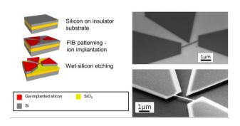
**Figure 1:** Left: definition of structures by means of Ga<sup>+</sup> ion implantation and subsequent wet etching of the silicon to form the final structure.
