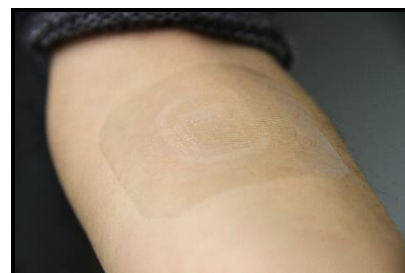
Figure 3: Photograph of the packaged image sensor.
