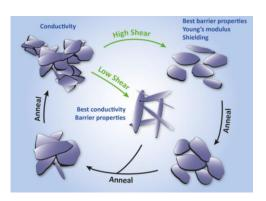
**Figure 1:** Schematic of processing effects on the GNP structure within the composite
