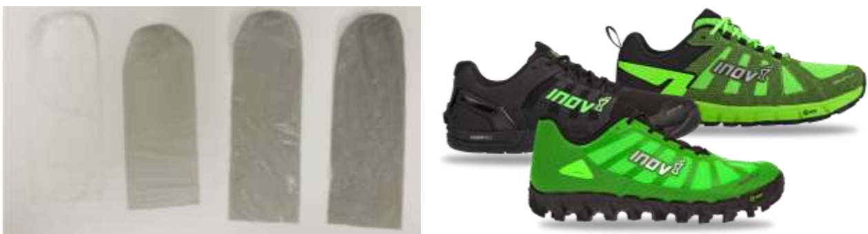
Figure 1: (a) Dip-molded graphene-elastomer thin film samples with increasing graphene content ((Left to right). (b) Graphene-rubber composite sole footwear (Inov-8 Ltd.).
