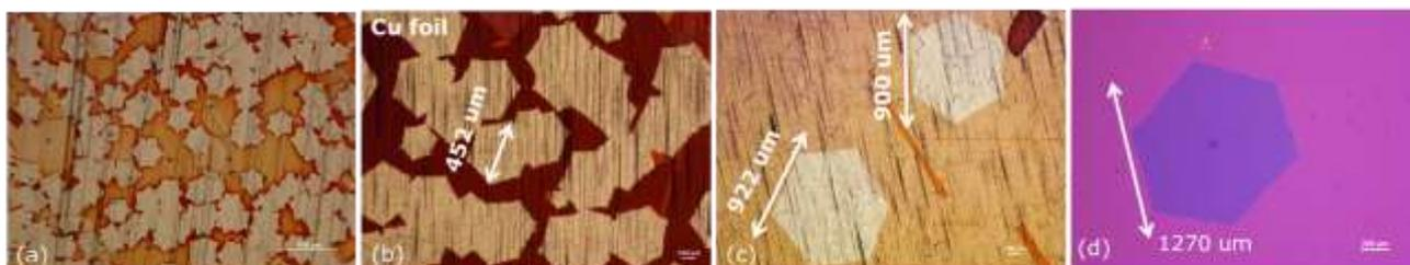
**Figure 1:** (a) Graphene grown by conventional CVD method. (b) Cu surface pre-treatment in  $\text{FeCl}_3/\text{HCl}$  solution. About 600 nuclei/cm<sup>2</sup> can be achieved. (c) Large graphene single crystals through a height-confined graphite reaction cavity (d) As-transferred millimeter size graphene single crystal.
