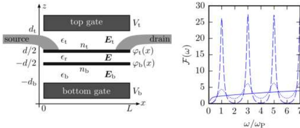
**Figure 1:** Schematics of the double-gated bilayer graphene setup (left) and photoresponse as a function of the driving frequency (right) for several carrier densities  $n = 0.1$  (solid),  $1.0$  (dotted), and  $5.0$  (dashed)  $\times 10^{12} \text{ cm}^{-2}$ .
