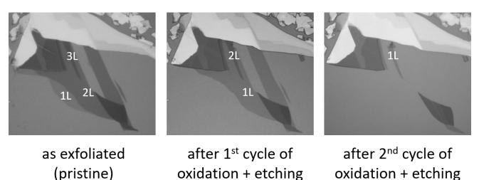
Figure 1: Optical images show clear demonstration of repeatable atomic-layer etching with monolayer precision
