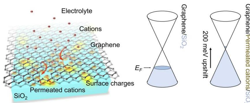
**Figure 1:** Illustration of cation permeation through the graphene sheet to the graphene- $\text{SiO}_2$  interface. Graphene is initially hole-doped due to the presence of negative surface charges (indicated in yellow) on the  $\text{SiO}_2$  surface. Intercalated cations lead to a shift of the Fermi level of graphene toward the Dirac point.
