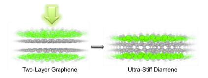
**Figure 2:** DFT simulations of the transformation of two-layer graphene into diamene under pressure.
