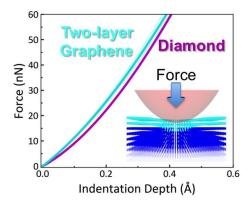
Figure 1: Experimental load vs. indentation curves showing that two-layer epitaxial graphene is stiffer than diamond.
