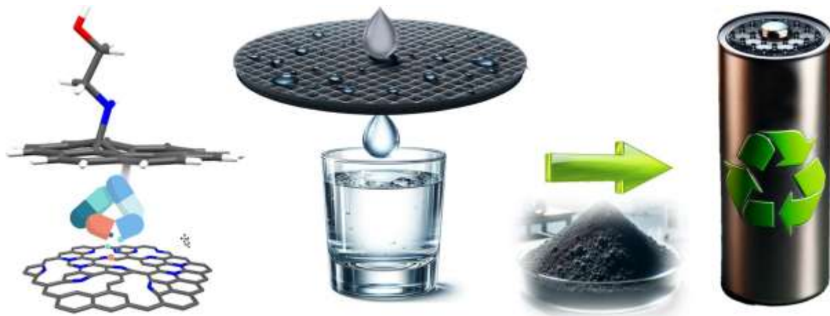
Figure 1: After removing pharmaceuticals from water, spent graphene-based sorbents are repurposed into redox-active supercapacitor electrodes.
