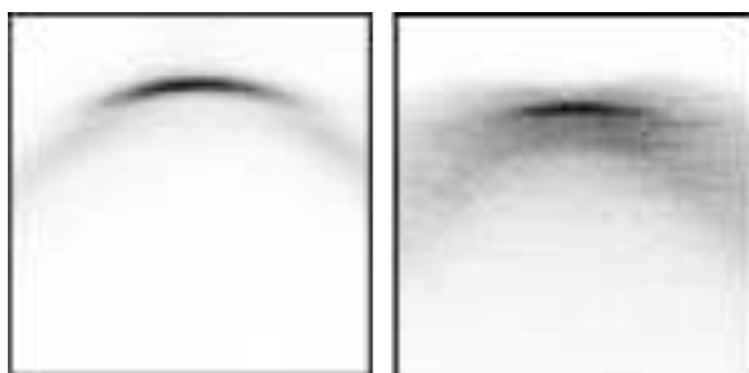
Figure 1: Electronic structure of K-point of exfoliated monolayer hBN (left) and bulk hBN (right).
