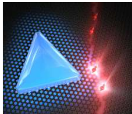
Figure 1: Left: realization of an altermagnet on graphene, with four H atoms on alternating sublattices. Right: inducing both superconductivity and magnetism in graphene generate exotic Yu-Shiba-Rusinov states, a starting point to ultimately create graphene topological qubits.
