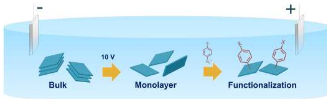
Figure 1: One-pot exfoliation-functionalization protocol used in this work.
