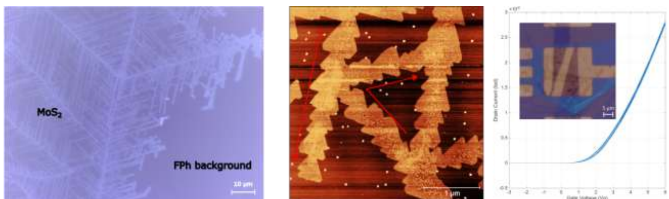
Figure 1: (A) Optical image of MoS 2 grown on the FPh substrate. (B) AFM image of MoS 2 ribbons, demonstrating the jagged nature of the growth as well as the growth direction of the ribbons (red arrows). (C) Transfer curves of a transistor fabricated from a MoS 2 ribbon, using hBN as the dielectric (device optical image shown in the inset).
