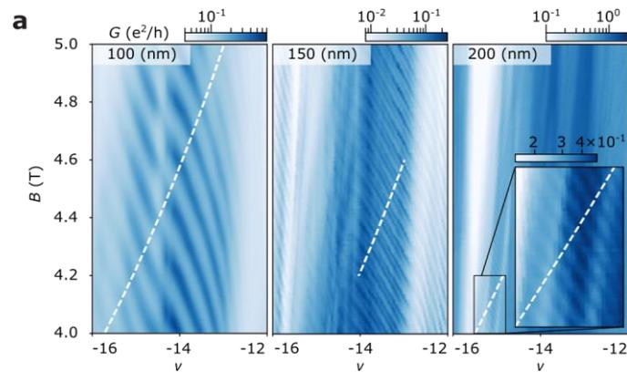
**Figure 2: Scaling with contact size.** Left to right: Two-terminal conductance measured as a function of the filling  $\nu$  and the magnetic field  $B$  with contact radius 100 nm, 150 nm and 200 nm.
