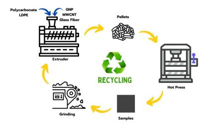
Figure 1: Recycling process for polycarbonate
