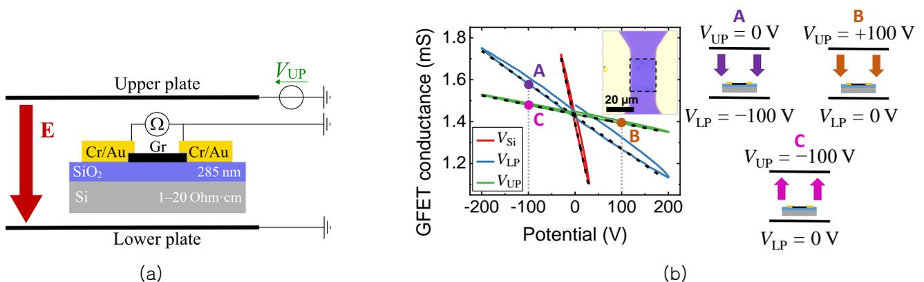
**Figure 1:** (a) Schematic representation of the graphene field-effect transistor in the test bench composed of two metallic plates facing each other to generate an electric field. (b) Graphene drain-source conductance as a function of silicon potential (red), lower plate potential (blue) and upper plate potential (green). The inset shows an optical microscope image of the graphene strip. On the right, configurations corresponding to the points A, B and C.
