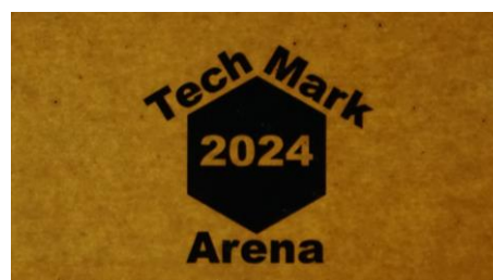
Figure 1: Laser-induced graphene (black area) in a lignosulphonate, cellulose, boron nitride coating.
