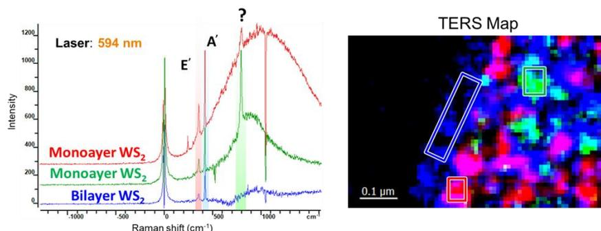
**Figure:** TERS spectra (left) averaged from a hyperspectral map (right) of WS<sub>2</sub>@1L h-BN@Au.
