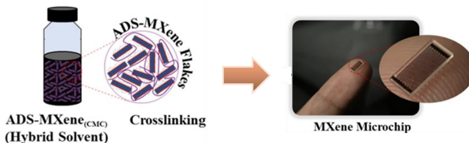
Figure 1: MXene microchip fabricated via EHD printing with ADOPA-functionalized MXene
