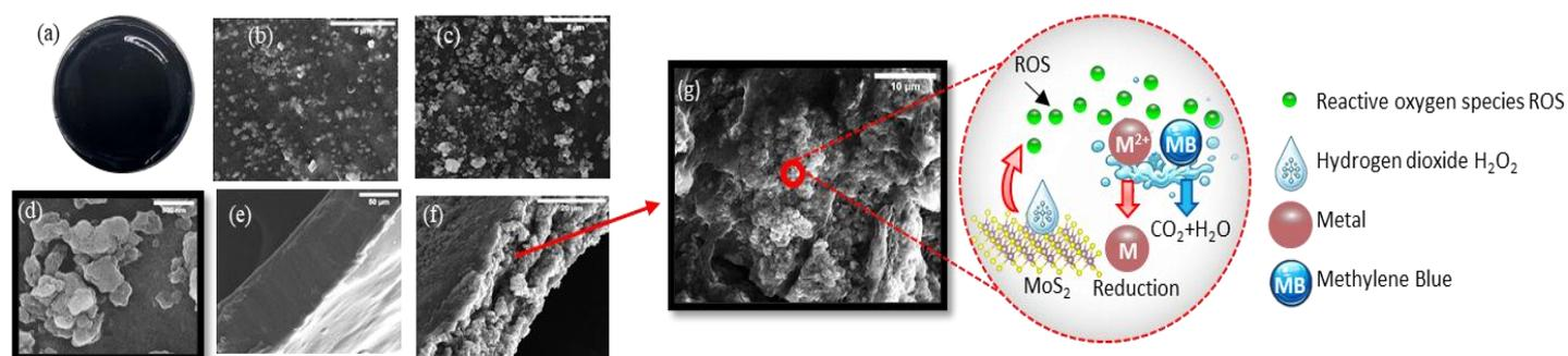
**Figure 1:** (a) Fabricated membrane, SEM images: (b) Base, (c) Top surface, (d) Top surface Magnified View, (e) Cross-sectional view of neat Membrane, (f) Cross-sectional view of fabricated membrane, (g) Magnified view of fabricated membrane.
