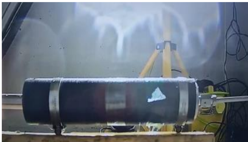
Figure 1: Illustration of tubular structure hydrodynamic burst test conducted.
