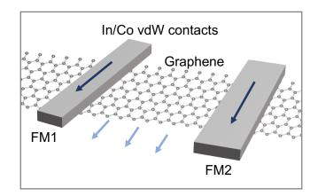
**Figure 1:** Schematic of a graphene lateral spin valve with ferromagnetic van der Waals contacts that can enable room temperature spin injection without dielectric tunnel barriers.
