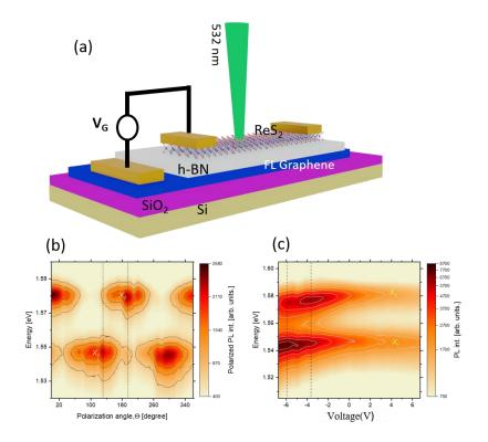
Figure 1 (a) Schematic of device used for gate voltage dependent polarization studies of  $ReS_2$ . (b) Polarization dependent PL of  $ReS_2$  at 5K. (b) Gate tunable PL of  $ReS_2$  shows that at large negative bias, X<sub>1</sub> quenches and emission becomes dominated by X<sub>2</sub>
