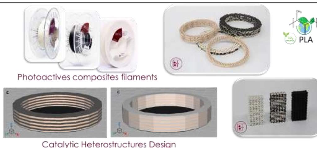
Figure 1: Example of a self-supported heterostructure based on MTE in water treatment for functional filaments based on titania and graphene nanoparticles.
