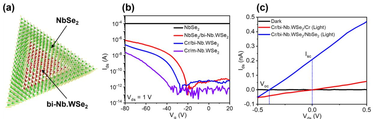
**Figure 1:** (a) Schematic illustrating the CVD growth of NbSe<sub>2</sub>/bi-Nb.WSe<sub>2</sub> heterostructure. (b) Transfer characteristics of Cr/m-Nb.WSe<sub>2</sub> (purple line), Cr/bi-Nb.WSe<sub>2</sub> (blue line), NbSe<sub>2</sub>/bi-Nb.WSe<sub>2</sub> (red line) and Cr/NbSe<sub>2</sub> (black line) contact FETs. (c) Output characteristics under dark and light conditions for Cr/bi-Nb.WSe<sub>2</sub>/Cr and Cr/bi-Nb.WSe<sub>2</sub>/NbSe<sub>2</sub> devices.
