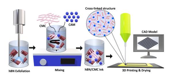
**Figure 1:** 2D hBN/CMC Composite Ink Formulation with citric acid monohydrate (CAM) as cross-linker and 3D printing process of model generated using a Computer-aided design (CAD) software [1]
