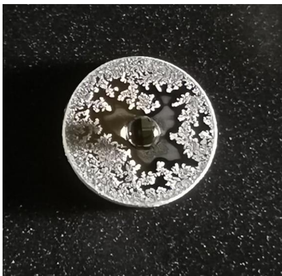
Figure 1: Water droplet on graphene, still liquid at -26.8°C.
