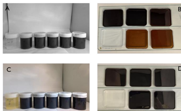
Figure 1: Sample A & C mixture solution GO/PVA & rGO/PVA with different molecular weight PVA polymer and sample B & D fabrication of GO/PVA & rGO/PVA films.
