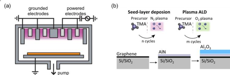
**Figure 1:** (a) A side view schematic of Atomfab's plasma source [patent application PCT/GB2019/052763]. (b) Process scheme of AlN seed-layer deposition and Al<sub>2</sub>O<sub>3</sub> plasma ALD.
