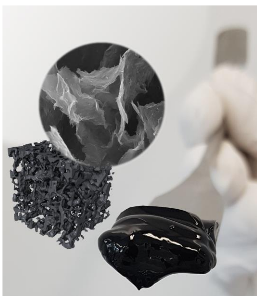
Figure 1: Aggregated graphene nanosheets are processed into a homogeneous gel that can be used for formulation of additive-free functional inks.
