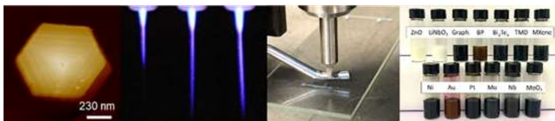
Figure 1: Examples of inks and printers for direct writing of electronics. Left to right shows thermoelectric flakes, plasma jet printing, aerosol jet printing, and library of developed inks.
