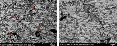
lifetime, reducing costs for maintenance and replacement. **Figure 1:** SEM images showing (left) GCuW contact surface and (right) CuW contact surface after single 5 kA shot, with some remaining W grains indicated.
