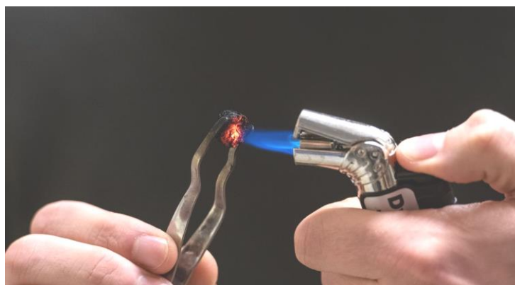
Figure 1: Flame-resistance testing of a cellular graphene aerogel using a propane flame.
