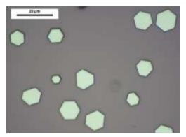
Figure 1: Optical image of Fe<sub>x</sub>Se<sub>y</sub> on SiO<sub>2</sub>
