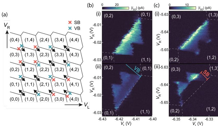
**Figure 1:** (a) Schematic charge-stability diagram for bilayer graphene double quantum dots at zero magnetic field, where blue and red crosses at triple points label valley and spin blocked transitions. (b, and c) Finite-bias triangles at zero magnetic field with (i) positive, and (ii) negative source-drain bias V<sub>SD</sub>, around triple points with carrier occupancy (b): (0,2)↔(1,1) showing valley blockade, and (c): (0,3)↔(1,2) showing spin blockade.
