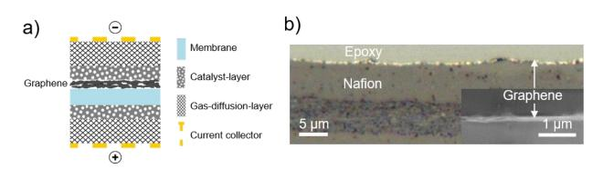
**Figure 1:** (a) Schematic of graphene-enhanced MEA. (b) Optical micrograph of graphene coated Nafion<sup>®</sup> membrane cross-section. Inset: STEM-ADF image of interface region.
