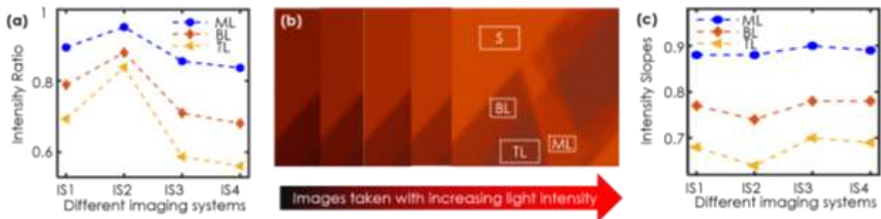
Figure 1: (a) & (c) Intensity ratio & slope of different layered regions (ML/BL/TL: mono/bi/tri-layer) from images of MoS 2 on 285nm SiO 2 /Si. (b) RGB images of MoS 2 flake (S, substrate) with increasing light intensities.
