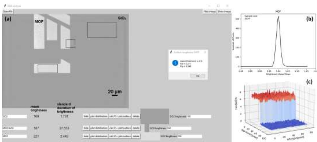
Figure 1: (a) Graphical user interface based on the developed analytical model for MOF thin films, inset shows thickness and surface roughness. (b) Brightness deviation of the selected region. (c) 3D projection for the selected region.
